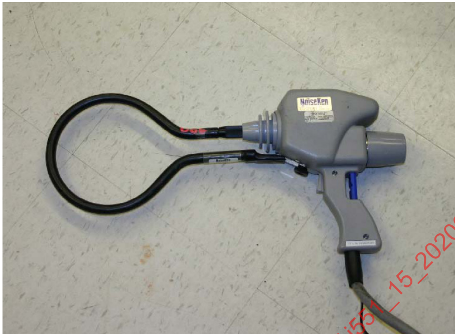
Figure 4 - An example of the magnetic field adaptor for rf impulse test
