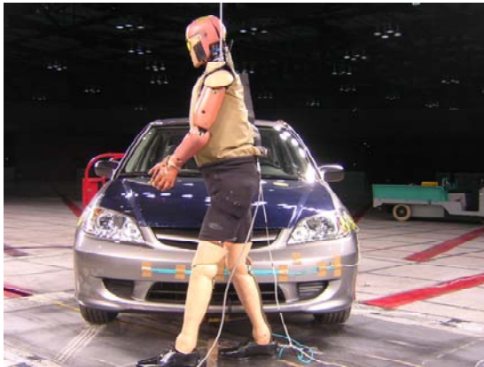
FIGURE D1 - TEST CONFIGURATION FOR POLAR II DURABILITY TESTING
