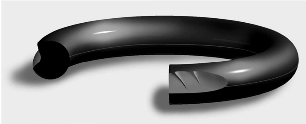
FIGURE 22 - INSTALLATION DAMAGE (USED WITH PERMISSION FROM R.L. HUDSON)
