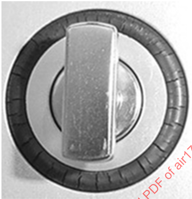
FIGURE 17 - CRACKING FROM OZONE
