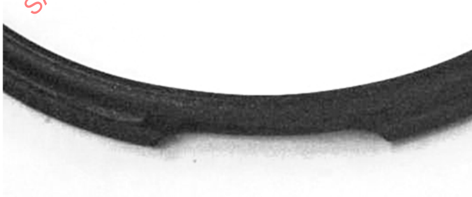
FIGURE 24 - SKIVED INSTALLATION DAMAGE
