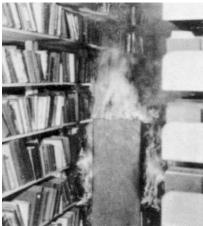
FIGURE J.3(b) After approximately 3 minutes; active burning in first tier; no sprinklers.
