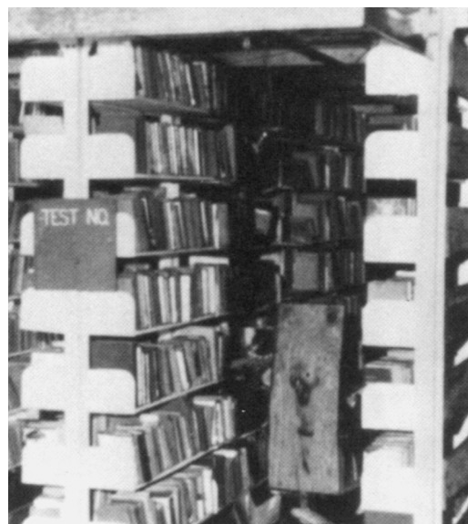
FIGURE J.2(f) Close-up of extent of fire damage after Test 1 with automatic sprinklers. Note limited area of fire damage.
