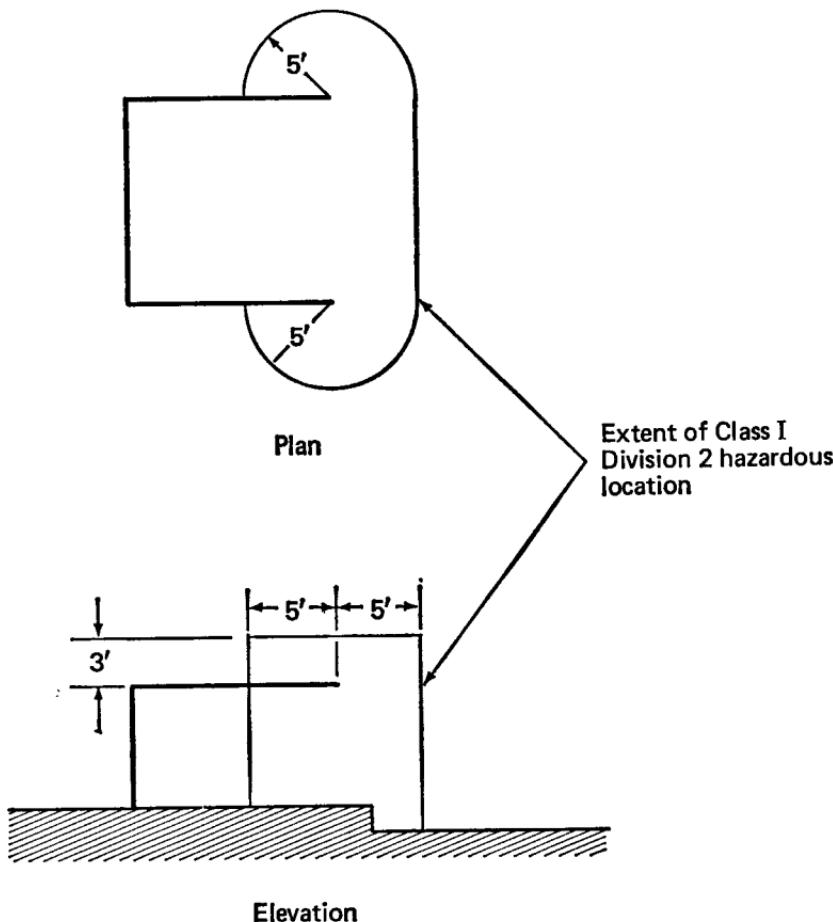
extend from the open face or open front of the spray booth or room in accordance with the following:
