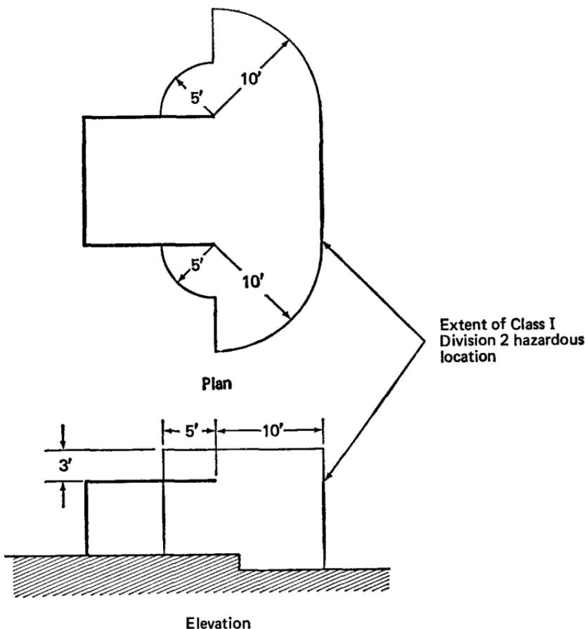
inoperable when the ventilation system is not in operation, the space shall extend ten feet from the open face or open front of the booth or room, and as otherwise shown in Figure 3.
