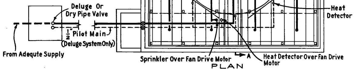
Figure 5-2c. Typical deluge or dry pipe fire protection arrangement for counterflow towers.
