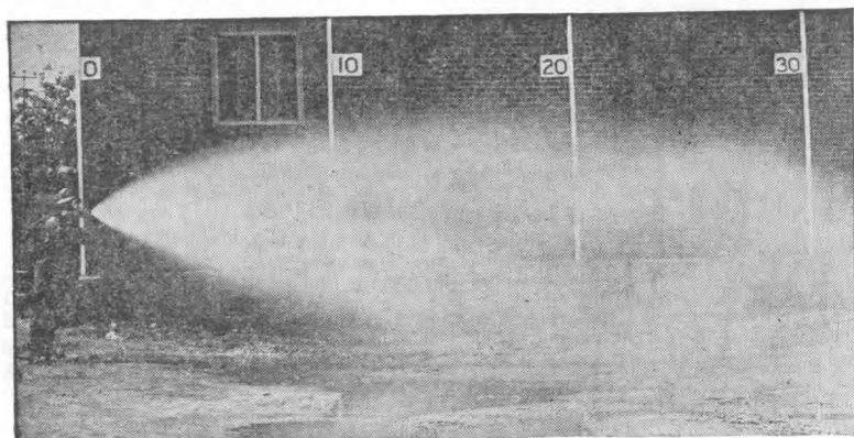
A11.30. A spray nozzle discharge showing the pattern of the spray. Numbers on wall indicate distance from nozzle in feet.
