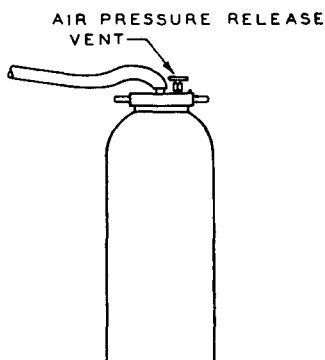
Figure A-5-5.3c. Hydrostatic Testing of Extinguisher with Test Bonnet.
