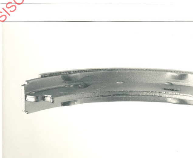
Figure 51 — Lining overhang on shoe platform edge
