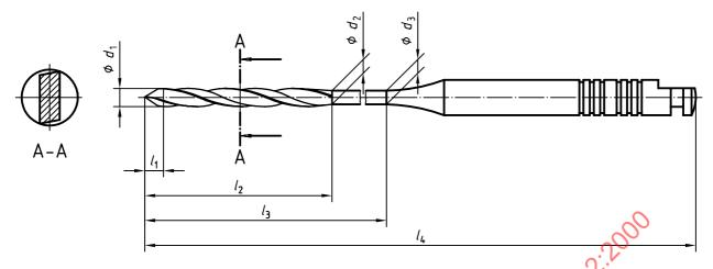
NOTE The shank shown is an example of type 1 of ISO 1797 with six-ring marking.
