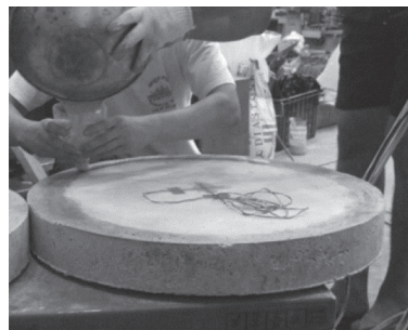
a) Capping and strain gages placed on the bottom of the test specimen
