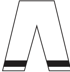
Figure 2 — Minimum pattern for placement of high-visibility materials on garments covering the lower torso including the legs (front and back)
