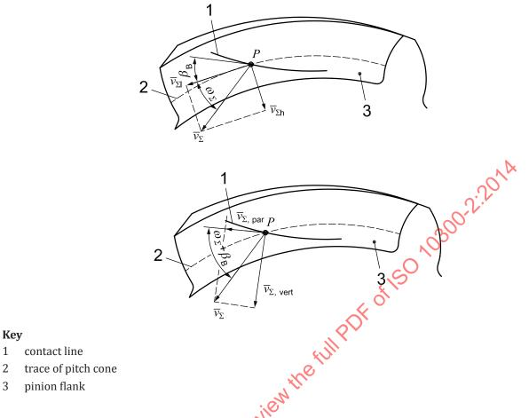
Figure 5 — Sum of velocities vertical and parallel to the contact line in the mean point P
