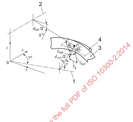
Figure 3 — Tangential velocities in the mean point P
