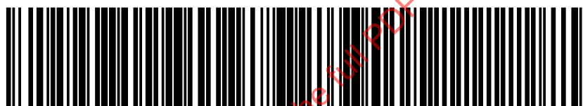
Figure 7 — Code 128 encoding “25SUN043325711MH8031200000000001”
