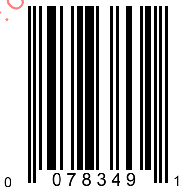
Figure 4 — UPC-E bar code symbol (encoding “0 07834 00009 1” by zero suppression). A UPC-E symbol implicitly encodes a digit zero (0) as a prefix to the GTIN-12 data structure.
