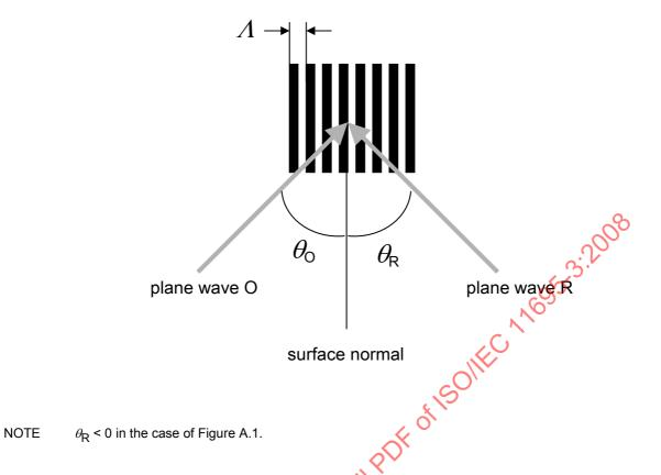
Figure A.1 — Recording of a diffraction grating in the storage layer by interference of two plane waves
