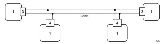
a) 2-WISE auxiliary device ports connected in parallel with short wires (stubs) to the cable
