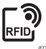
Figure 5 – Marking of a RFID transponder as a digital nameplate
