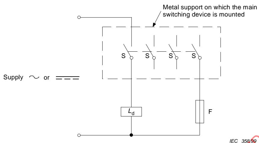
**Figure 2a – Contact elements of the same polarity, non electrically separated**
