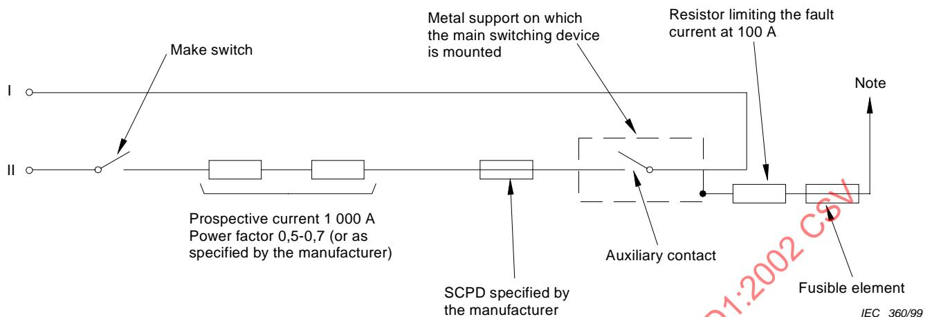
NOTE To be connected alternatively to I or II in successive tests.
