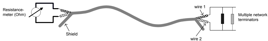
Figure N.5 – Resistance measurement between wire 1 and wire 2
